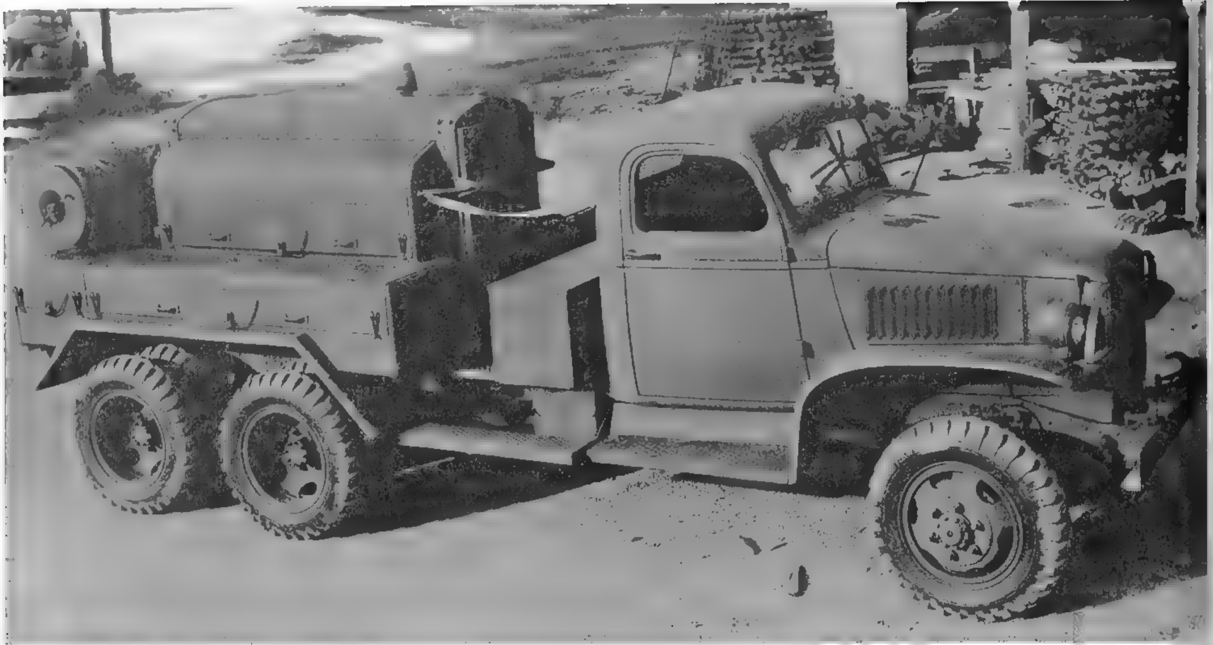
Certain Army Engineer units were provided with Le Roi air compressors mounted on CCKW chassis. Both open- and closed-cab chassis were used. (Photo courtesy of U.S. Army Engineer School History Office)
